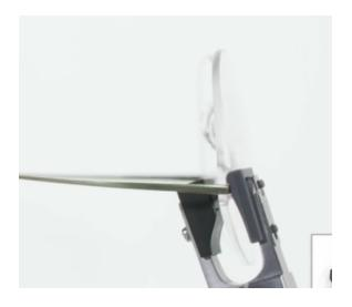
Support temple and lens mounting with mounting pliers to prevent stress on lens mounting
